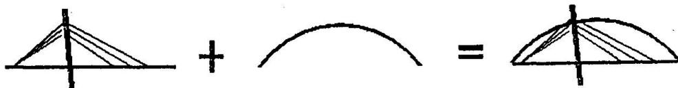
Fig. 9 A new bridge type by adding an arc to a cable-stayed bridge
