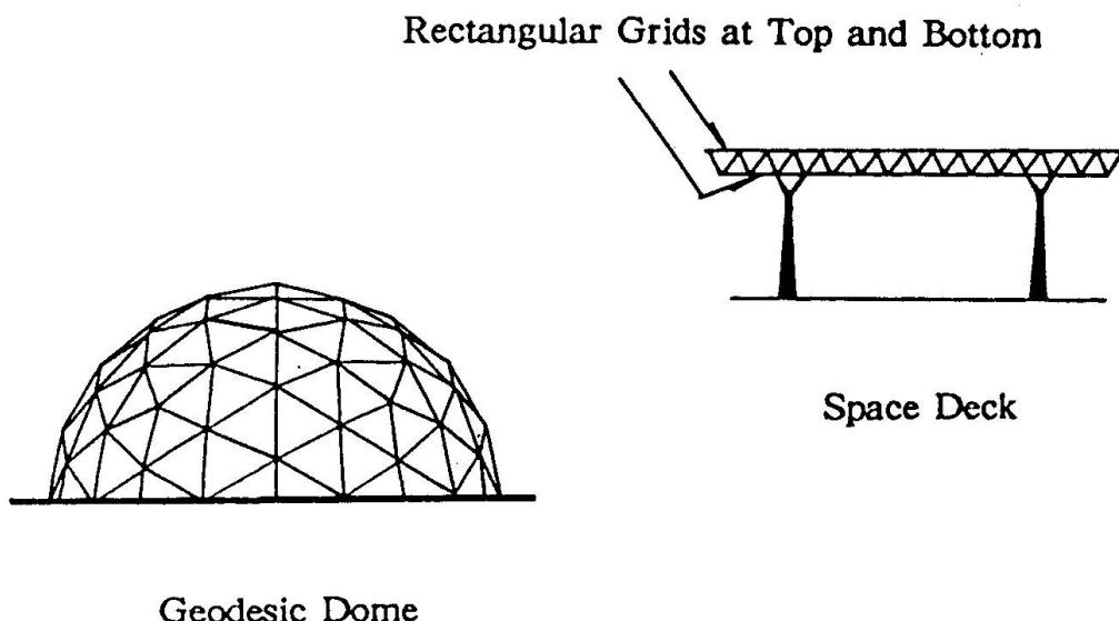
**Fig.1** Typical spatial grid structures
