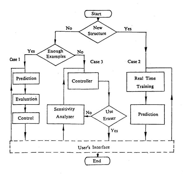
Fig.2 System architecture of SPRED-2
