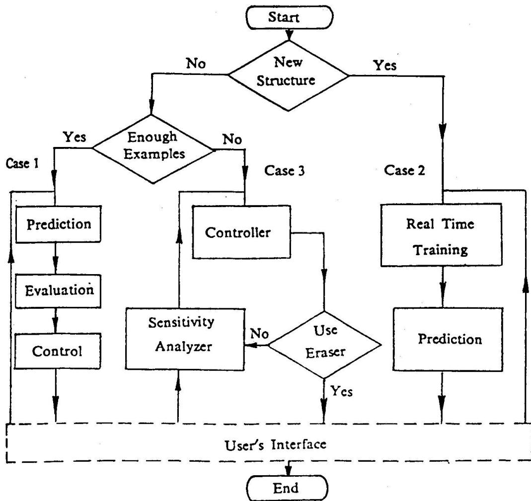
**Fig.2** System architecture of SPRED-2
