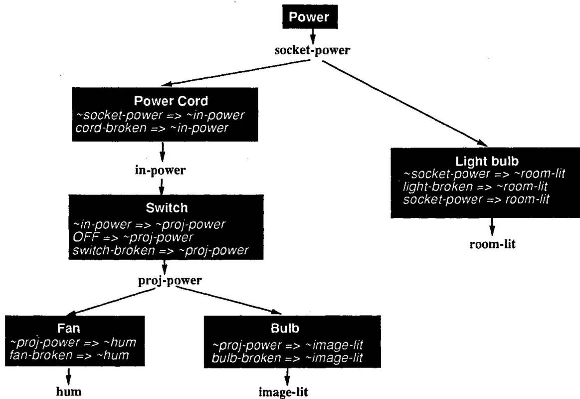
Figure 1: Models used for diagnosing a projector.
