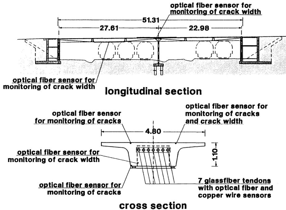
Figure 5: Measurement layout
