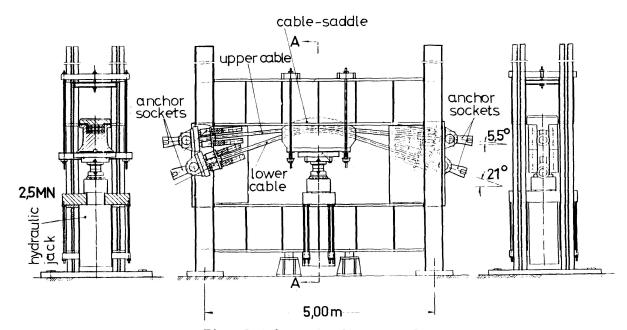
Fig. 3 Schematic diagram of test set-up
