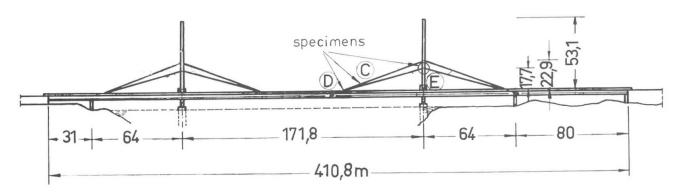
$\frac{\text{Fig. 5}}{\text{5}}$  Schematic diagram of the Norderelbebridge with the points where the specimens were drawn from
