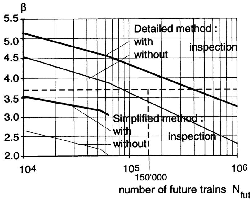
Figure 2 Reliability index for chord member 18/19 as a function of the number of future trains for simplified and detailed probabilistic approach
