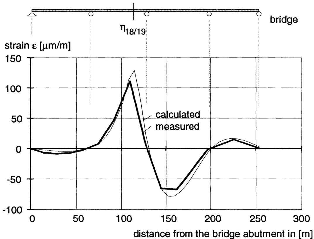
**Figure 4** Comparison between calculated and measured influence lines for bottom chord member 18/19 due to the passage of the engine. (The stress values are evaluated from the strain readings using an elastic modulus of 200'000 MPa.)
