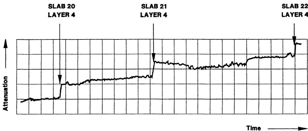
**REACTION OF THE CRACK - WIDTH SENSORS ON REMOVAL OF
