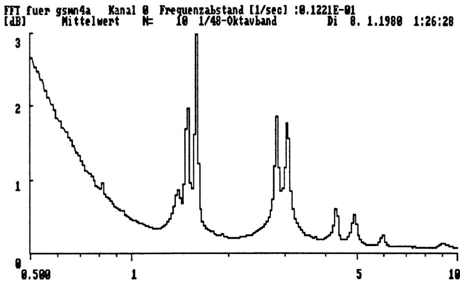
fig. 11 Averaged banded frequency spektrum at point N4
