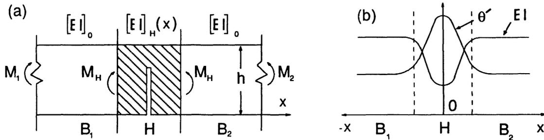
Fig.2 (a) Moments  $M$  and stiffnesses  $EI$  in cracked sections  $H$  and sound segments  $B$
