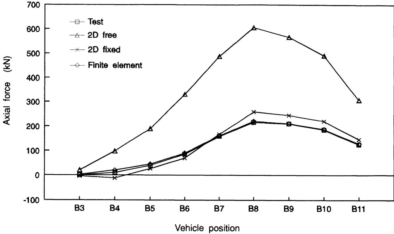
Fig. 3 Axial forces in the bottom chord
