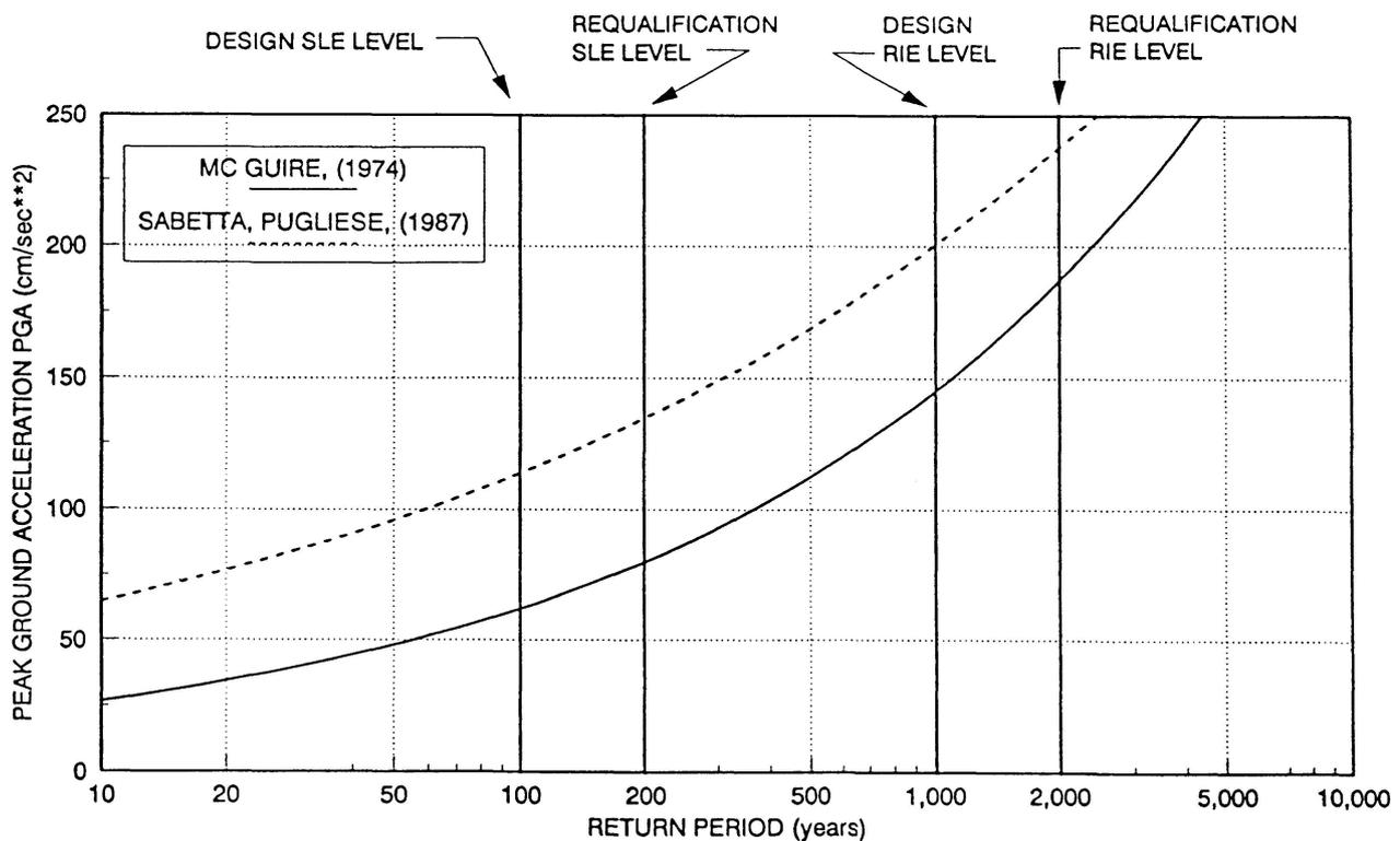
Fig. 3 Peak Ground Accelerations obtained adopting design and re-qualification attenuation laws
