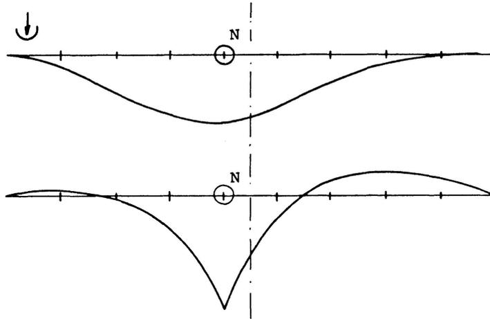
fig. 9 Static influence line of deflection and moment at point N4 calculated with finite elements method.
