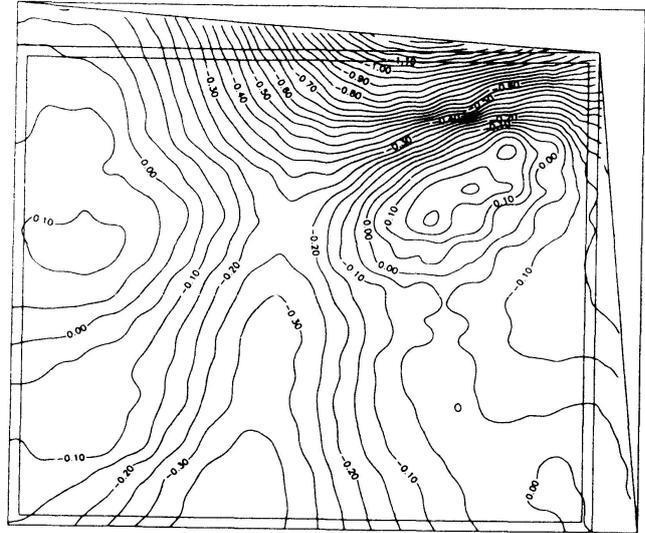
Fig. 6 Vertical deflection in shell at ultimate load for NLG analysis with prestressing.
