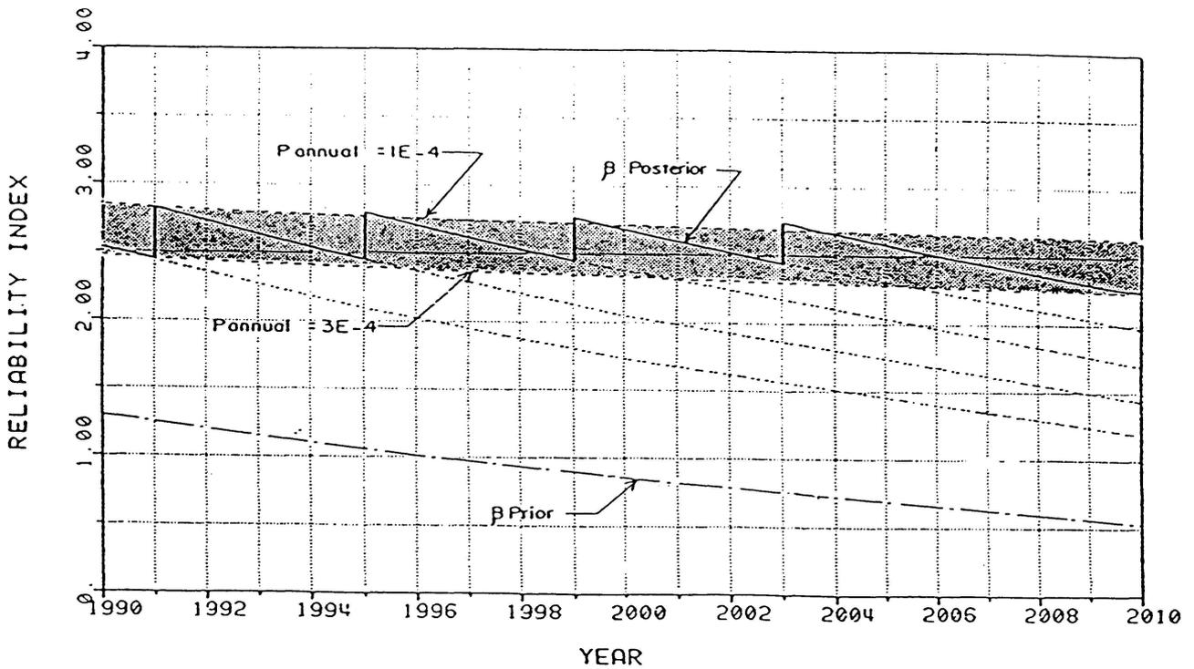
Fig 2 Reliability index vs. time and recommended inspection program.
