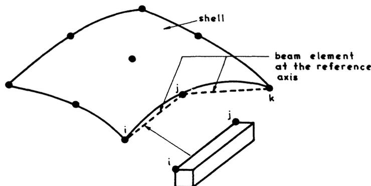
Fig. 3. Adopted L7 shell and straight beam elements
