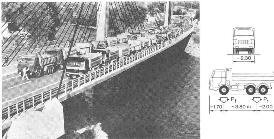
Fig. 1: Static load test of the Chandoline Bridge. The nominal dimensions of the lorries used for the load testing of bridges are also shown:  $P_f = 60$  kN,  $P_r = 190$  kN,  $P_{total} = 250$  kN
