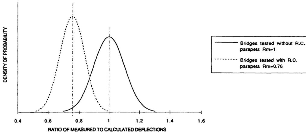
Fig. 6: Normal probability distribution curve for the ratio of measured to calculated deflections for bridges tested with and without R.C. parapets ( $E_c = 33.5$  GPa)
