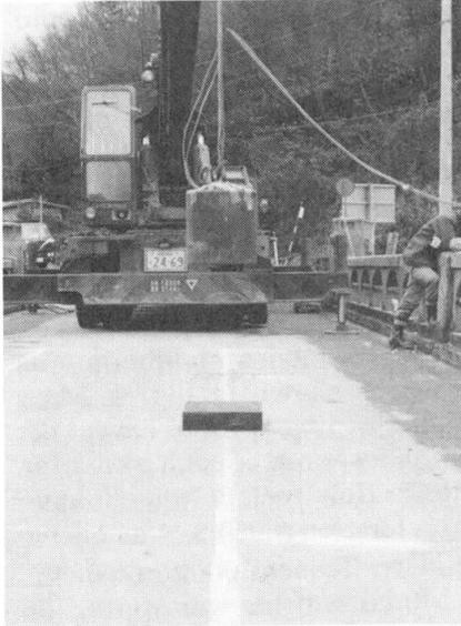
Fig. 4 Details of falling mass (dynamic) test
