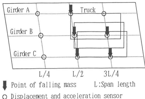
Fig. 3 Example of loading points and arrangement of sensors for static and dynamic tests
