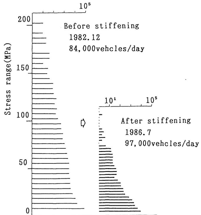
Fig. 4 Stress range histograms measured before and after the stiffening
