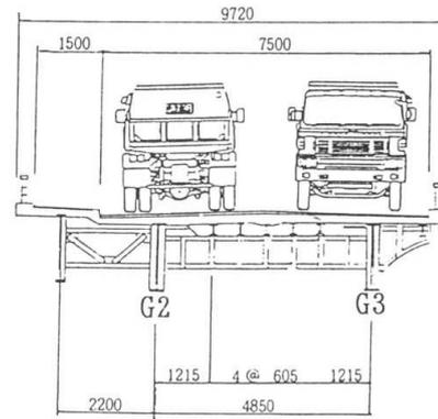
Fig. 3 Cross section of investigated bridge
