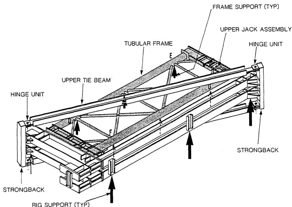
**Fig. 1** Frame test general arrangement
