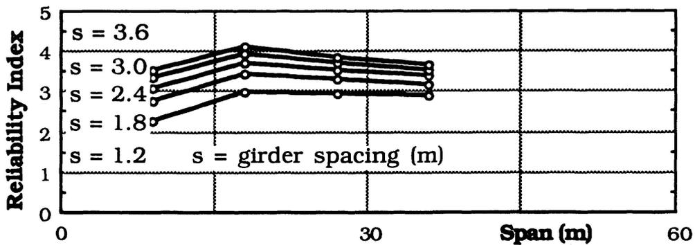
Fig. 3 Reliability Indices for Reinforced Concrete T-beams.
