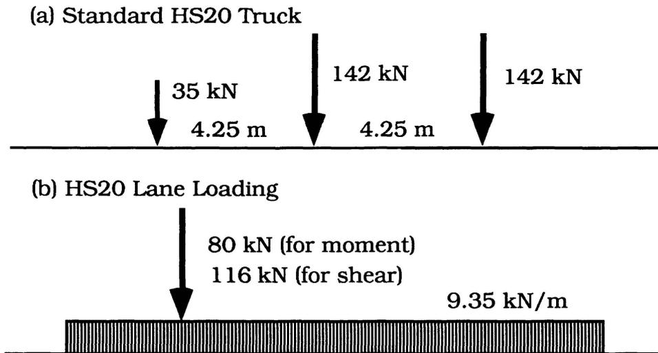
Fig. 1 AASHTO Standard Truck and Lane Loading [1].
