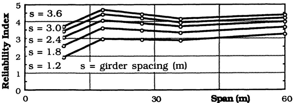
Fig. 4 Reliability Indices for Prestressed Concrete Girders.
