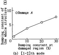
Fig.8 Damping characteristics
