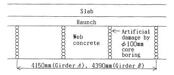
Fig.6 Inducement of artificial damage
