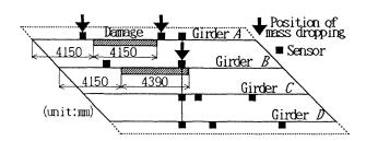
FIg.5 Outline of dynamic loading test
