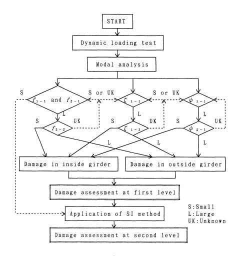
Fig.10 Flow of damage detection
