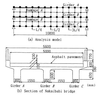
Fig. 1 Modeling of existing RC-T beam bridge
