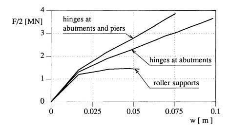
Figure 5 Influence of boundary conditions on load-bearing capacity.
