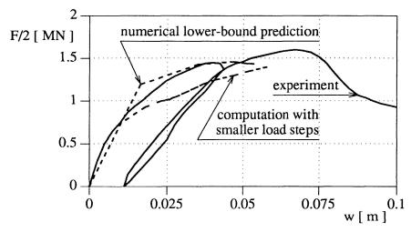
Figure 7 Numerically obtained lower-bound solution and the experimental failure load.
