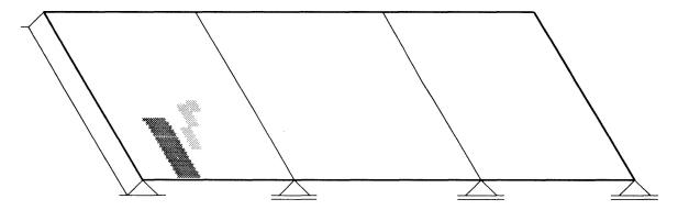
Figure 8 Spread of zone in which the bottom reinforcement is yielding at F/2 = 1.40 MN. The lighter shaded area has experienced less plastic flow.
