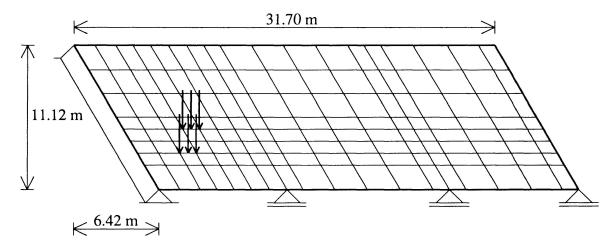
Figure 3 Finite element model for the Delft FE analysis of the bridge and position of the loads.
