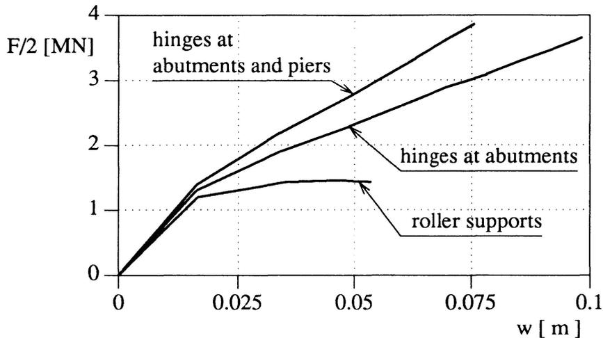
Figure 5 Influence of boundary conditions on load-bearing capacity.
