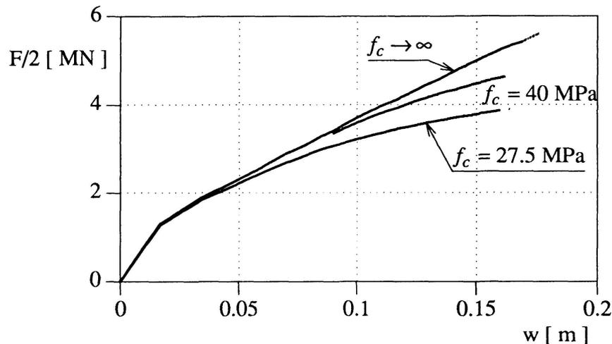
Figure 6 Influence of concrete plasticity on failure load for the case that there are hinges assumed at the abutments and roller supports at all piers.
