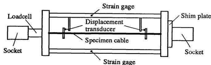
Fig.1 Measurement System
