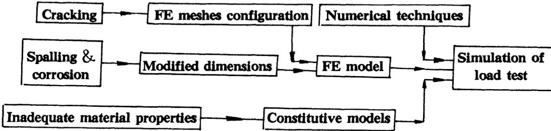
Fig. 2 Management of the factors affecting load capacity
