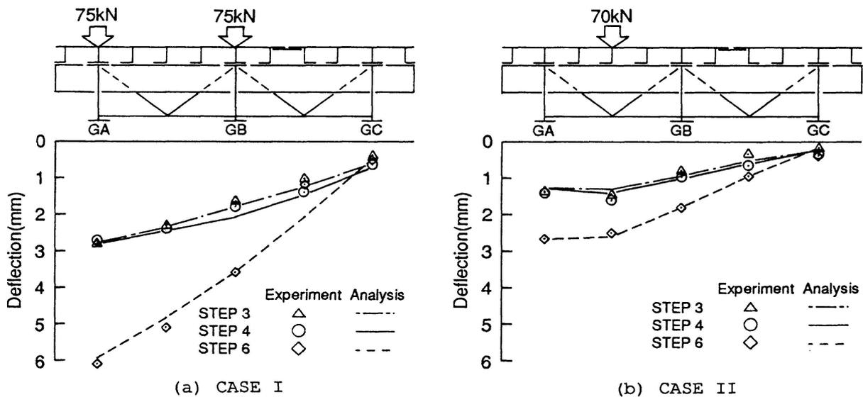
**Fig. 8** Comparison of deflection at midspan between theory and experiment
