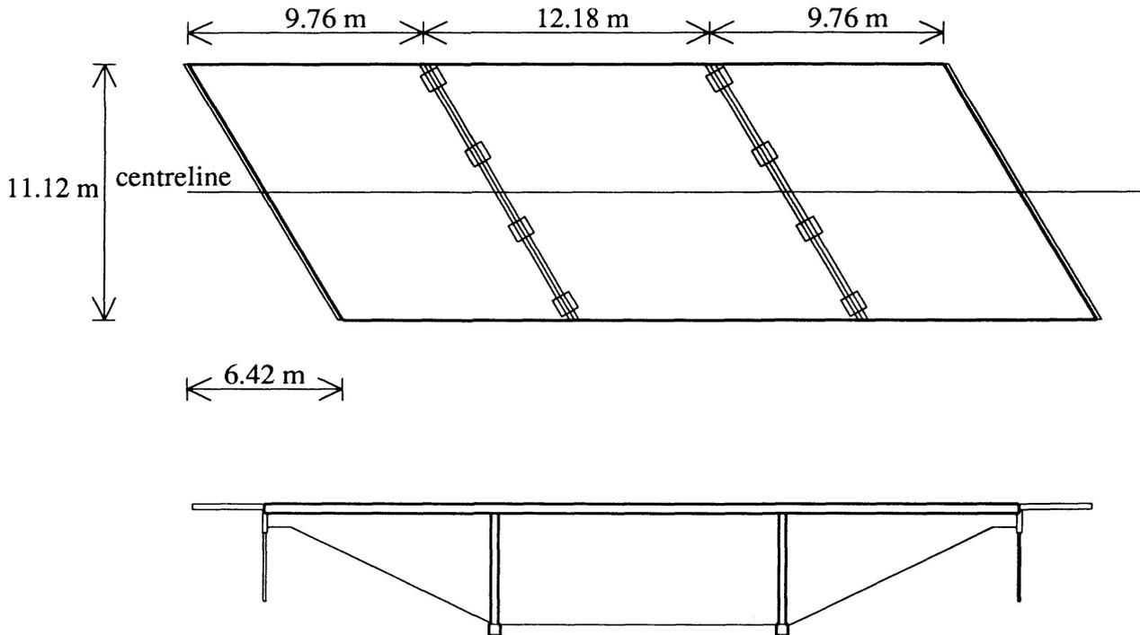
Figure 1 Plan view and side view of the bridge.
