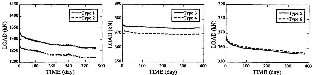
Fig.2 Time Variation of Cable Tensile Force
