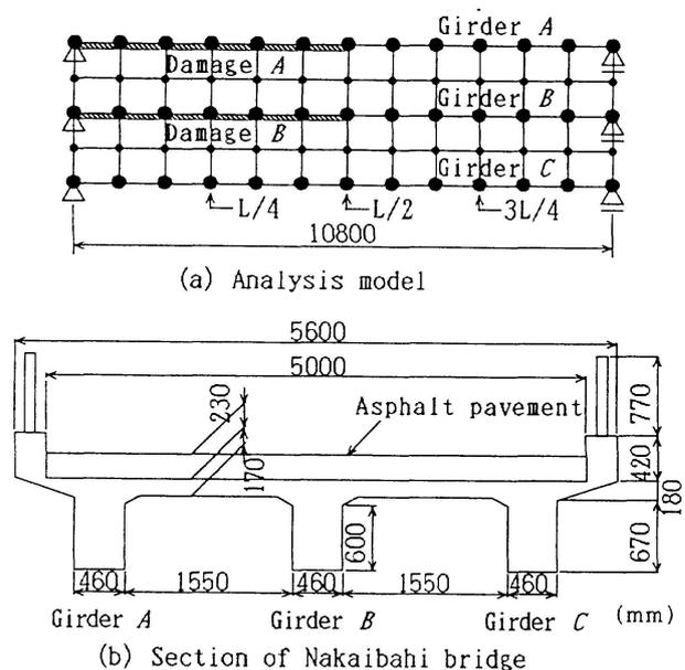
Fig.1 Modeling of existing RC-T beam bridge
