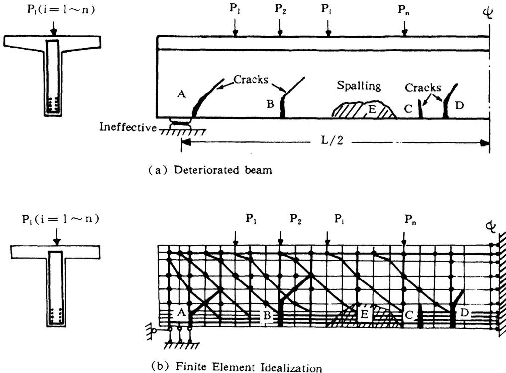
Fig. 3 Finite element model of deteriorated beam
