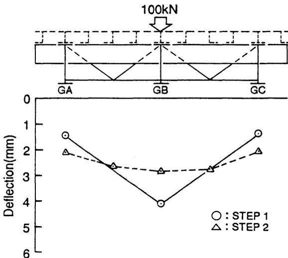
Fig. 4 Deflection of main girders at midspan
