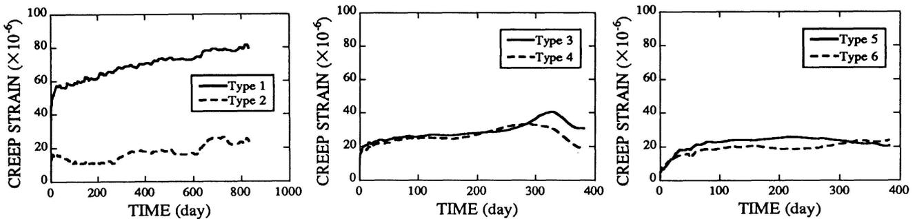
Fig.3 Time-dependent Behavior of Cables
