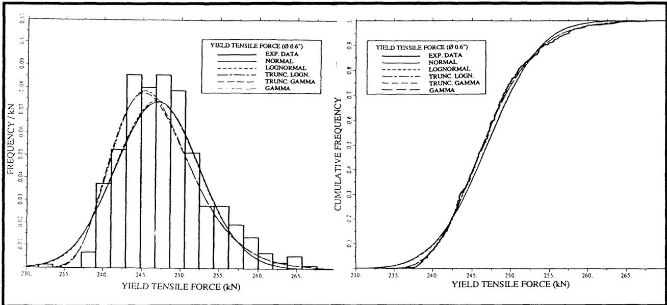
Figure 1.- Histogram, PDF and CDF curves, for yield tensile force prestressing steel. (strand 0.6")
