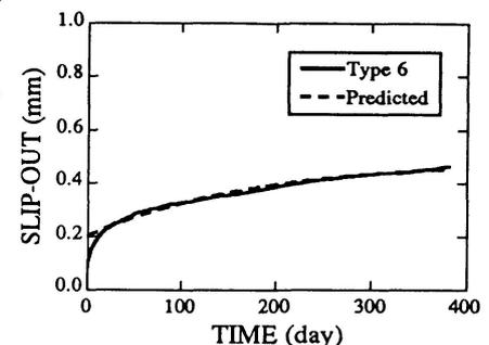
**Fig.9** Predicted Time-dependent Behavior of Sockets (Method 3)
