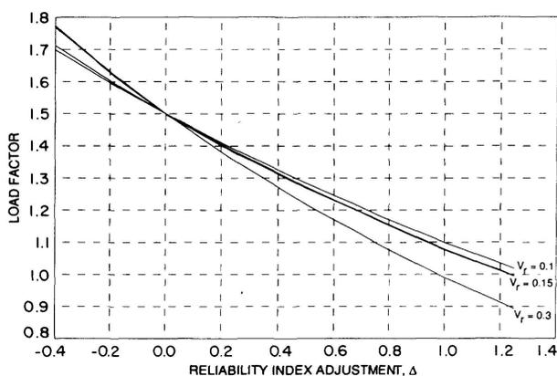
**Fig. 2** Variable Load Factor ( $V_S=0.3$ )
