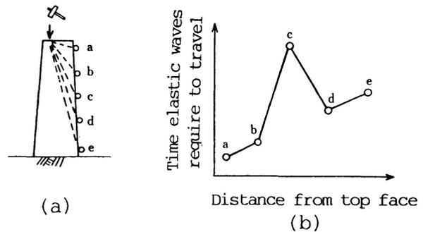
Fig. 9 Time-Distance Curve
