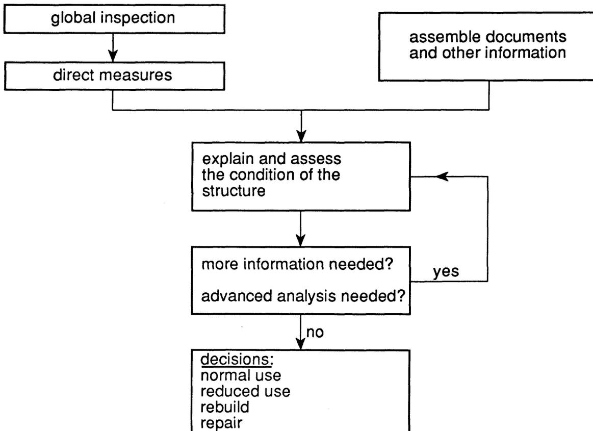
Figure 3: Event tree for a structure subject to a long term inspection and repair program; after every inspection the structure may be o.k. or need repair; during the inspection intervals the structure may fail
