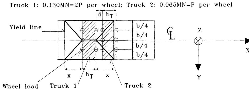
Figure 2. Yield line pattern in upper bound calculation.
