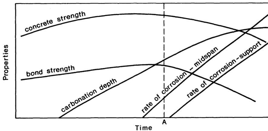
Fig. 4 Schematic change in element characteristics with time
