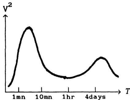
Wind loads are applied as pressures on structures. The pressure is proportional to the square of the wind velocity. The conventional wind velocity is measured at 10 m above the ground level and increases with altitude. The peaks of the frequency spectrum are between 3 s and 10 mn and around 4 days. Because of the nonstationarity of the wind, the velocity is described by its mean values or maxima over 10 mn to 1 hr periods. These stationary periods correspond to the lower
