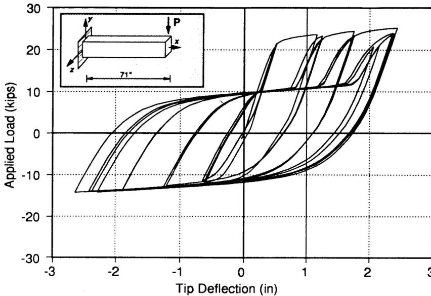
FIGURE 2 - TIP LOAD-DISPLACEMENT RESPONSE OF CANTILEVER BEAM UNDER CYCLIC UNIAXIAL BENDING
