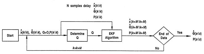
FIG. 2. The Adaptive Filter Procedure.
