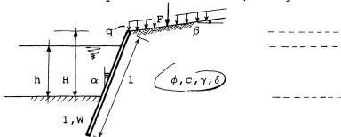
Fig.2 General sheetpiling wall
