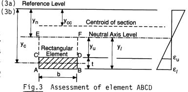
The axial force  $F_j$  supported by element j is given by the difference in axial forces on the two rectangles ABEF and CDEF:
