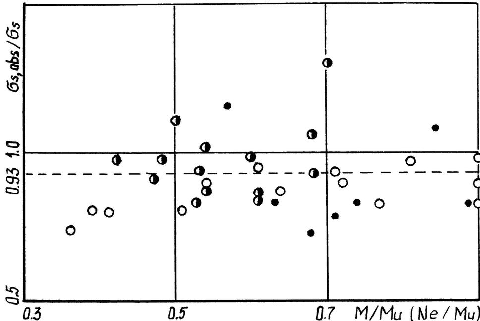
Fig.2 Comparison of measured in tests  $\sigma_{s,obs}$  and theoretical  $\sigma_s$  calculated by formula (11) tensile reinforcement stress values: ● - prestressed concrete beams; ○ - reinforced concrete beams; ◐ - eccentrically compressed members
