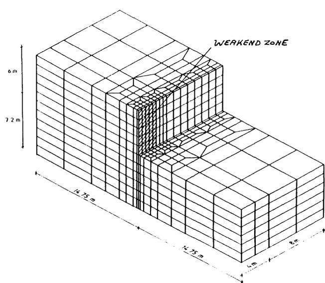
Fig.8 A 3-dimensional FEM-model of a sheetpiling wall.
