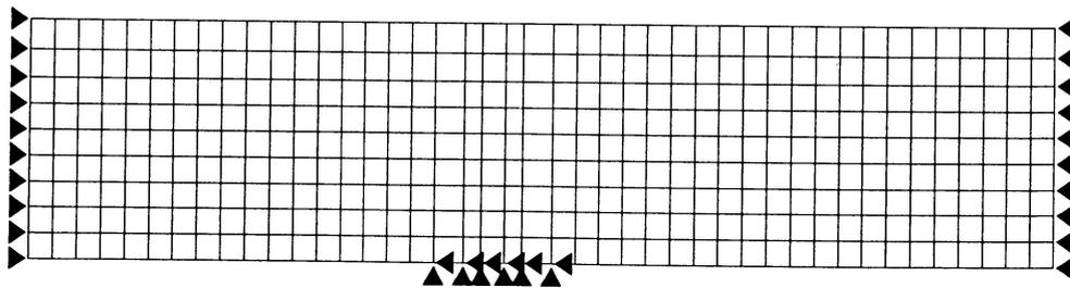
Fig.3 Finite element mesh of the structural model.
