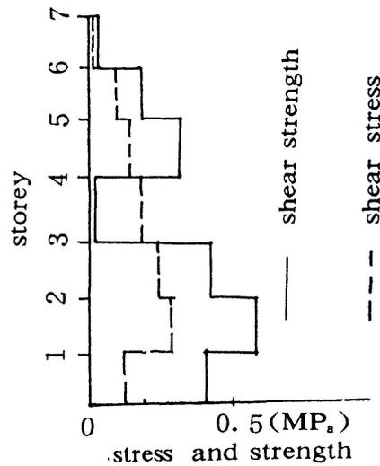
Fig. 4 Distribution of shear strength and stress
