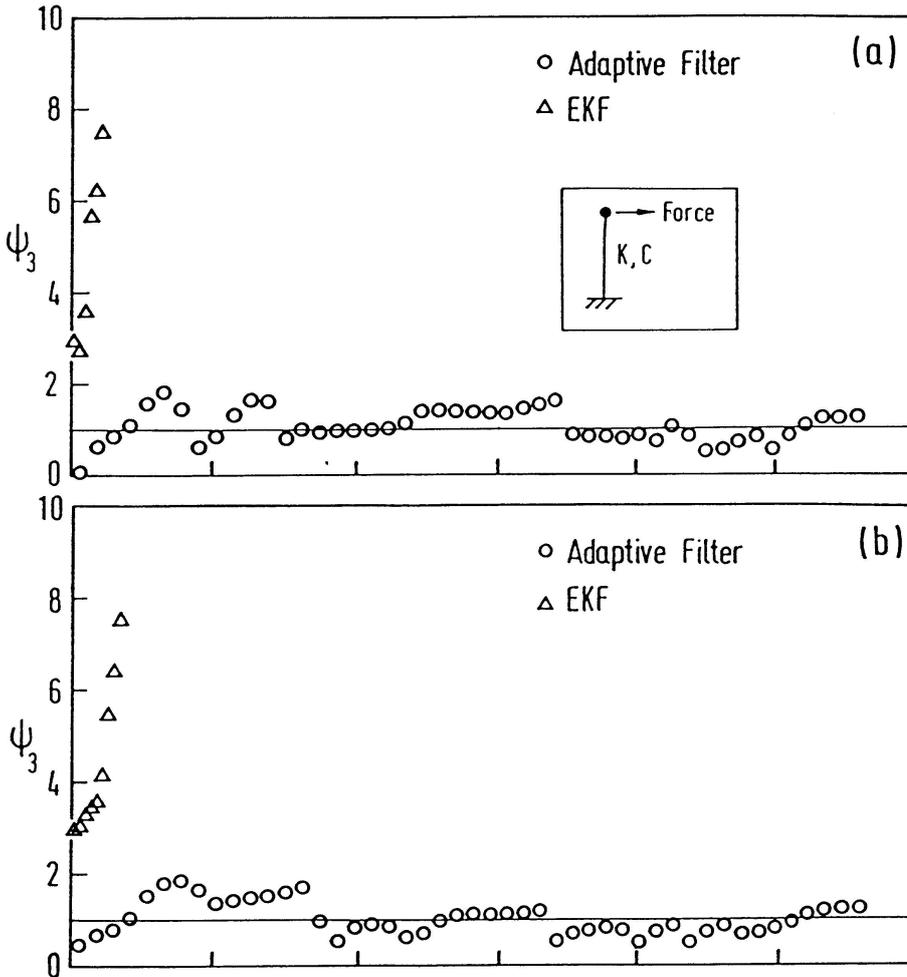
FIG. 3. Performance Indices for Stiffness (a) under 10% I/O Noise and (b) under 30% I/O Noise.
