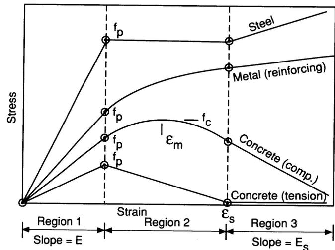
Fig.2 Stress-strain curves
