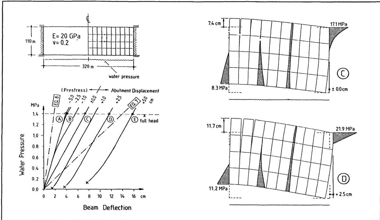
Figure 5: Hidden horizontal arch in a 'tension-free' beam
