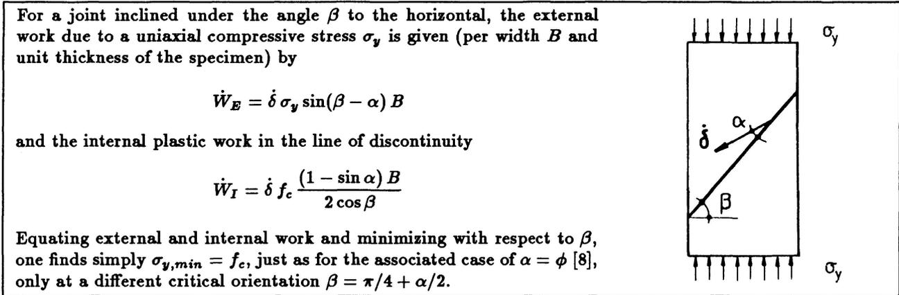
Figure 3: Analysis of a prism test with construction joint
