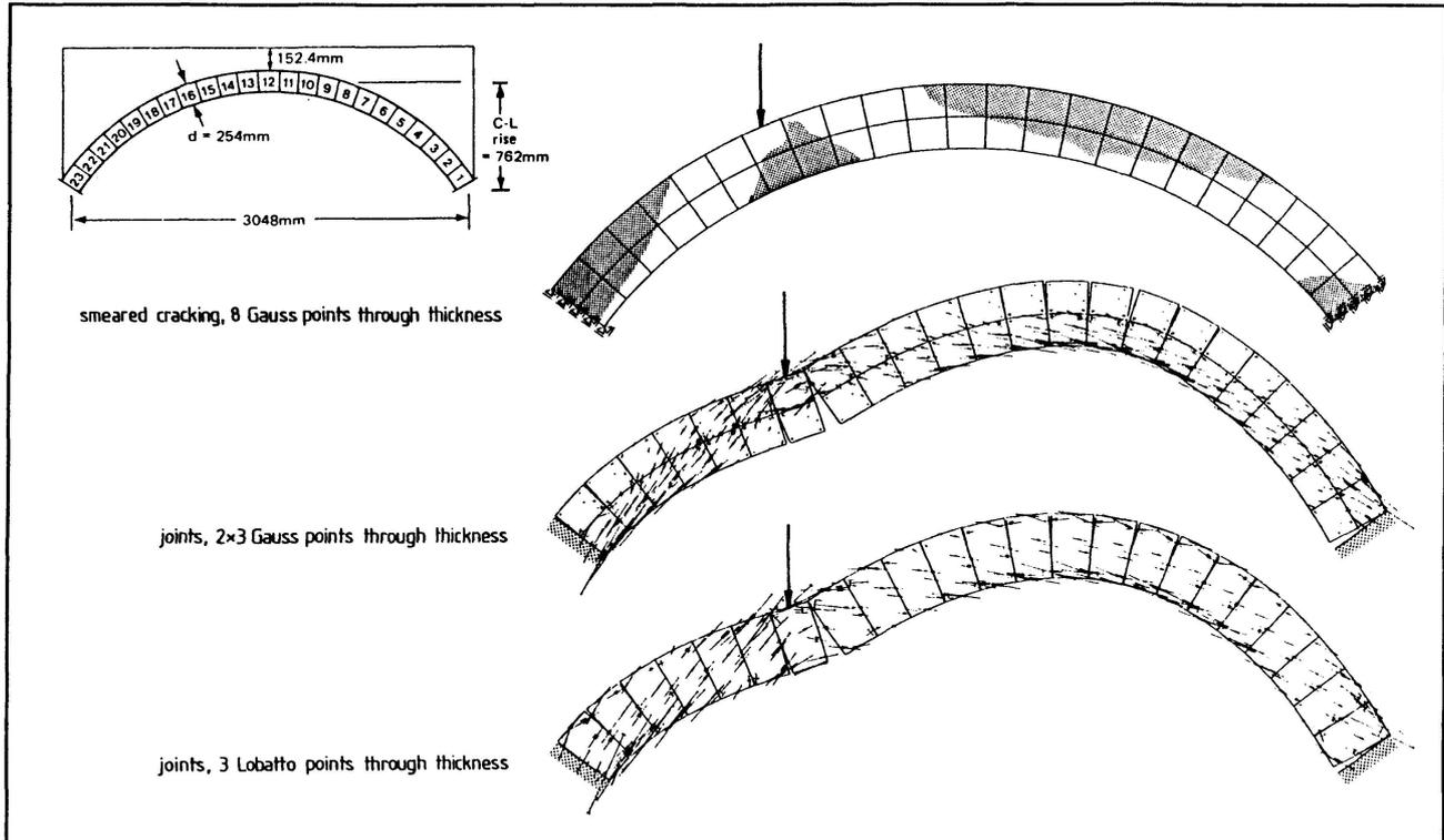
Figure 4: Discrete joint model of a circular arch
