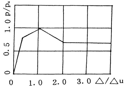
Fig. 1 Skeleton curve of masonry wall
