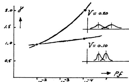
Fig. 6 Safety-factor vs. failure probability
