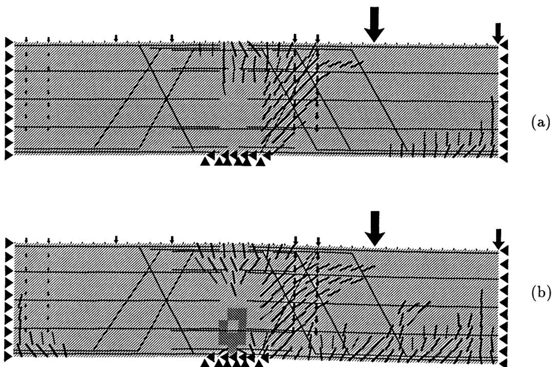
Fig.6 Comparison of damage states for cases of different joint concrete qualities.
