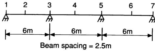
a) 3 - span beam : converted to continuous composite beam.
