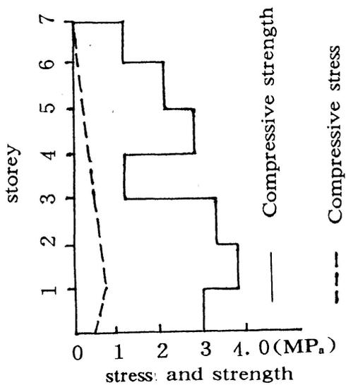
Fig. 3 Distribution of compressive strength and stress
