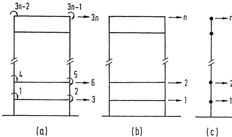
FIG. 1. (a) Complete Model; (b) Condensed Model; (c) Remedial model. (Numbers indicate DOFs).
