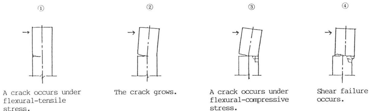
Fig.10 Failure Process [5]
