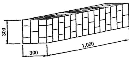
Fig. 5 Dimensions of Brick Specimen (unit: mm)
