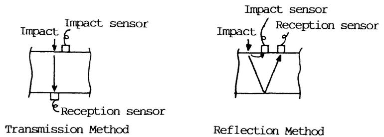
Fig. 4 Standard Measuring Method [4]
