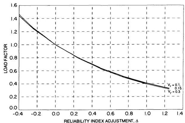
**Fig. 3** Earthquake load factor ( $V_S=1.1$ )
