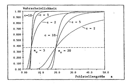
Fig. 2: Distribution function of the initial crack length for different parameter values, after Krä [15]
