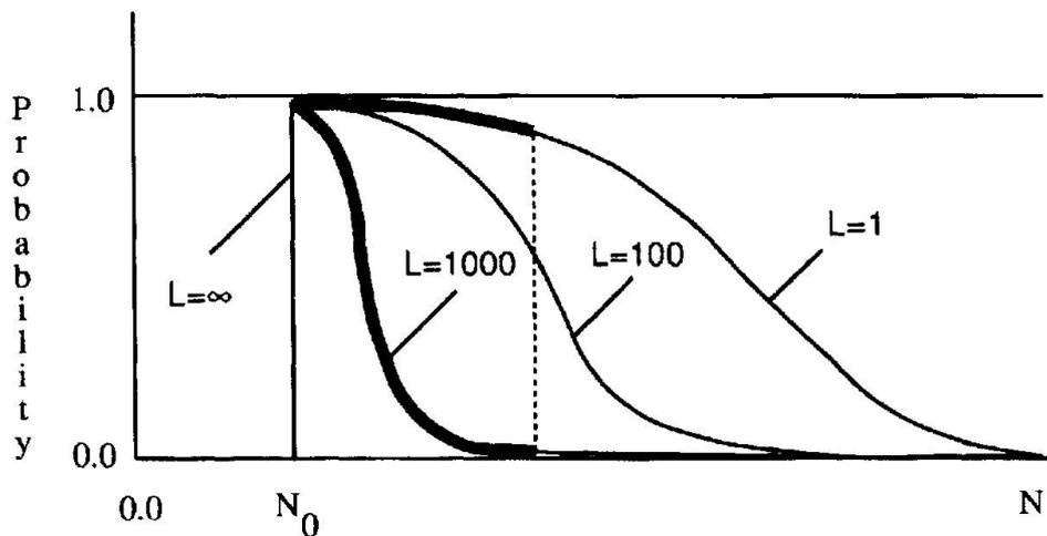
Figure 7: Survival function for different lengths 1, 100, 1000 and  $\infty$ .
