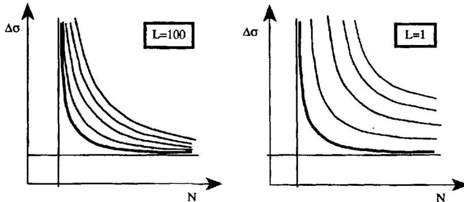
Figure 8: Whöler fields for two different lengths.
