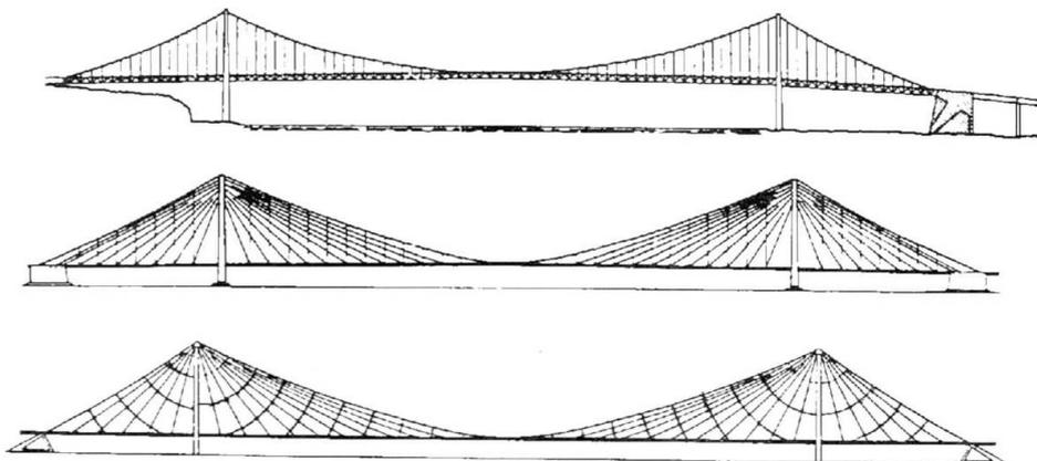
Fig.3 Loadbearing systems of large suspended bridges [1]
