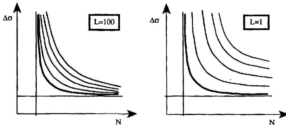
Figure 8: Whöler fields for two different lengths.
