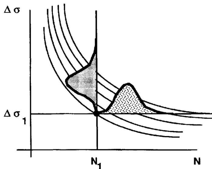
Figure 6: Two random variables:  $N$  for given  $\Delta\sigma$  and  $\Delta\sigma$  for given  $N$
