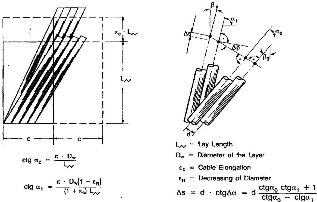
Fig.18 Relative movement  $\Delta s$  and rotation  $\Delta \beta$  of wires in stranded cables [43]
