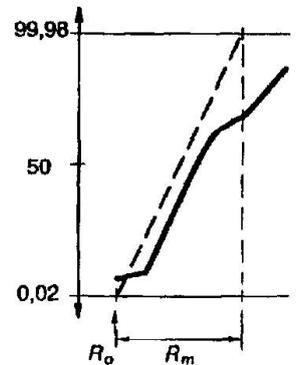
Fig.17 Statistic values of short specimen rupture tests (ϕ = 100mm) and fatigue tests (ϕ = 500mm) determined out of a special charge of these wires and strands
