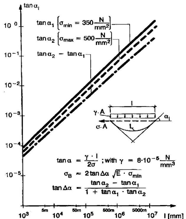
Fig. 20 The increase of the entry angle at the end of a cable, sagging under dead load, depending on the length if the cable-tension increases from 350 N/mm<sup>2</sup> to 500 N/mm<sup>2</sup>
