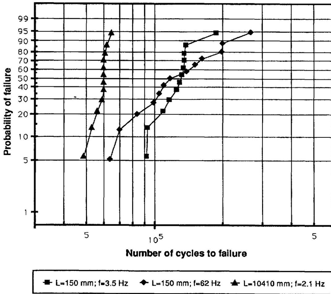
**Fig. 5: Fatigue of prestressing wires**
