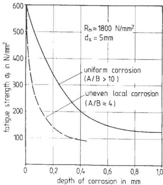
Fig.9 Fatigue strength under pulsating tensile stresses of corroded cold-drawn carbon steel wires (A=diameter of corrosion, B=depth of corrosion) (Neubert, Nürnberger) [24]
