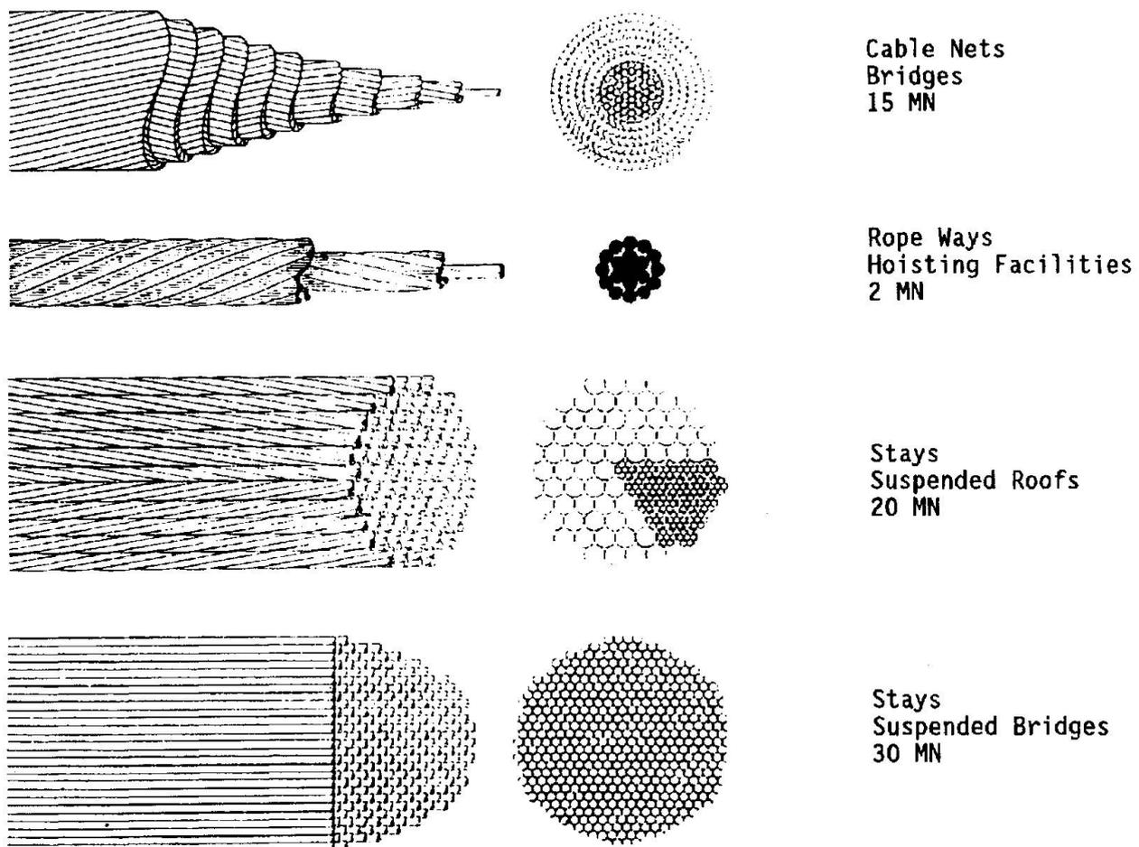
**Fig.1** Cross-sections of various cable-constructions and their fields of application
