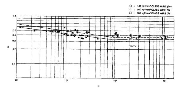
Fig. 3 S-N Curve of Galvanized Steel Wire
