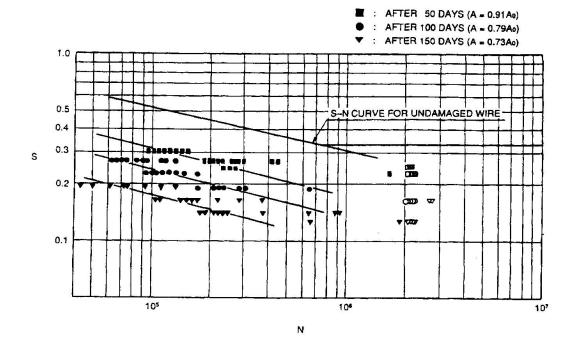
Fig. 7 S-N Curve of Galvanized Steel Wire after Salt Sprayed Test (Test Condition: 0.5 cm<sup>3</sup>/min., Salt Water (pH 6.5-7.2)) (Courtesy of Kobe Steel)
