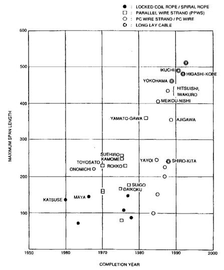
Fig.1 Historloal Change of Cable Type of Cable-Stayed Bridge in Japan
