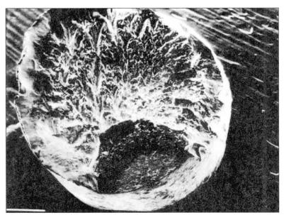
Fig 6 Fatigue fracture of 5mm wire.
