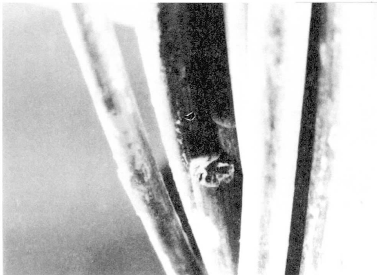
Fig 7 Fretting fatigue in 19-wire strand.
