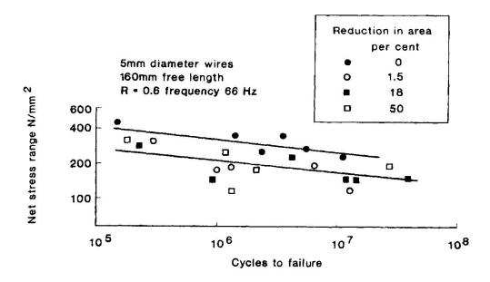
Fig.4 Endurances of corroded wires
