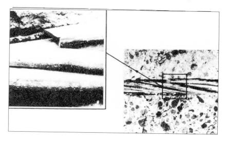
Fig 1 Fatigue fracture of prestressing strand in lightweight aggregate concrete beams.
