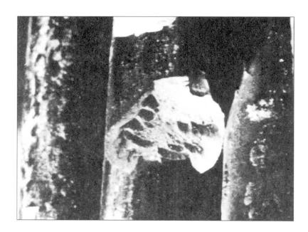
Fig 9 Initiation from corrosion pit in 19-wire strand.
