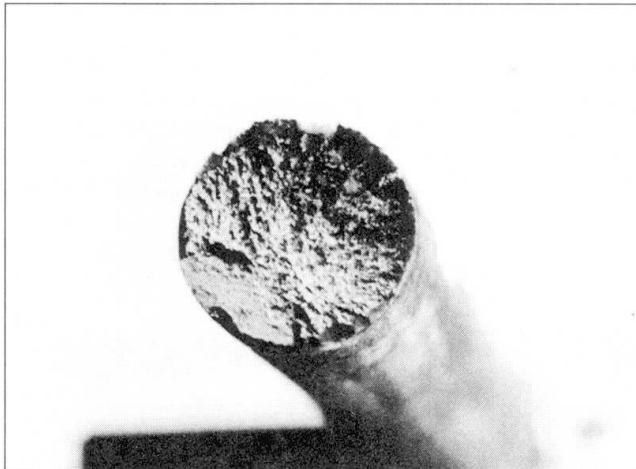
Fig 10 Initiation from corrosion pit in 8mm diameter wire.
