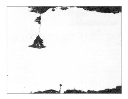
Fig 12 Corrosion fatigue crack adjacent to final fracture.
