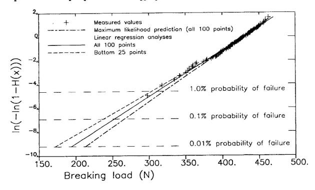
Fig. 3 Weibull plots of 100 yarn strength values measured by Amaniampong [10]
