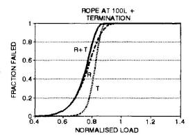
Fig. 5 Cumulative Weibull distributions, showing competitive failure of rope and terminations. For rope at length L,  $\alpha$  = 1 and  $\rho$  = 10. For termination,  $\alpha$  = 0.83 and  $\rho$  = 25. For rope at length 100L, calculation gives  $\alpha$  = 0.79 and  $\rho$  remains equal to 10.
