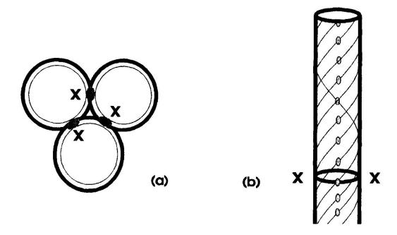
Fig. 4 Localised abrasion at contacts: (a) in cross-section; (b) along yarn
