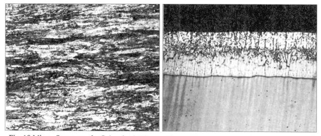
Fig. 10 Micro-Structure of a Galvanized Wire (400 Magnifications)
