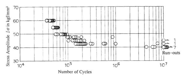
Fig. 9 Fatigue Test Result for 7 mm Dia. Galvanized Wire at a Mean Stress of 100 kgf/mm<sup>2</sup> (980 N/mm<sup>2</sup>)
