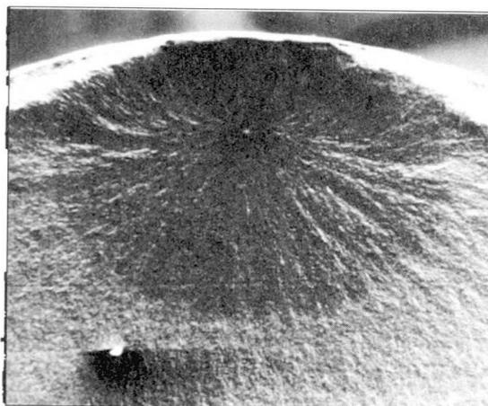
Fig. 7 Fatigue Fracture Surface of an OT Wire (50 Magnifications)
