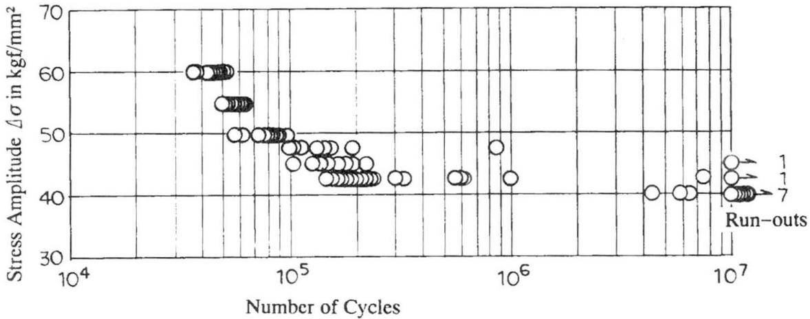
Fig. 9 Fatigue Test Result for 7 mm Dia. Galvanized Wire at a Mean Stress of 100 kgf/mm<sup>2</sup> (980 N/mm<sup>2</sup>)
