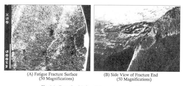
Fig. 4 An Example of Fatigue Failure of Prestressing Wire
