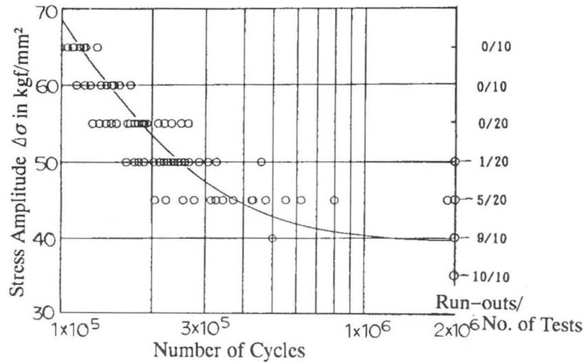
Fig. 3 An Example of Fatigue Test Results for a 7 mm Prestressing Wire
