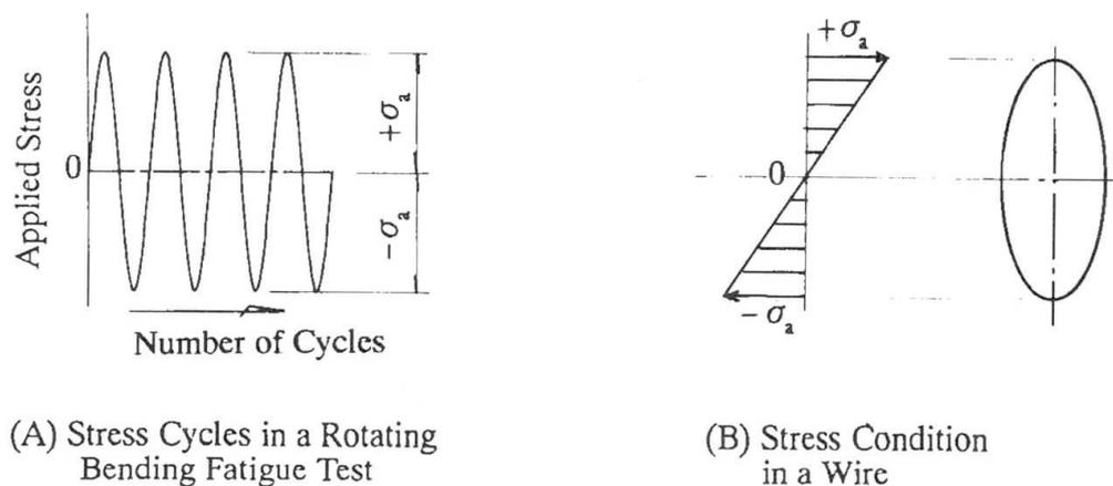
Fig. 5 Fatigue Test for Valve Spring Wire
