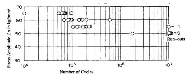
Fig. 8 Fatigue Test Result for 7 mm Dia. Galvanized Wire at a Mean Stress of 50kgf/mm<sup>2</sup> (490N/mm<sup>2</sup>)
