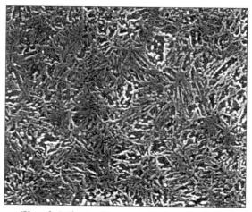
Fig. 6 Micro-Structure of an OT Wire (5,000 Magnifications)
