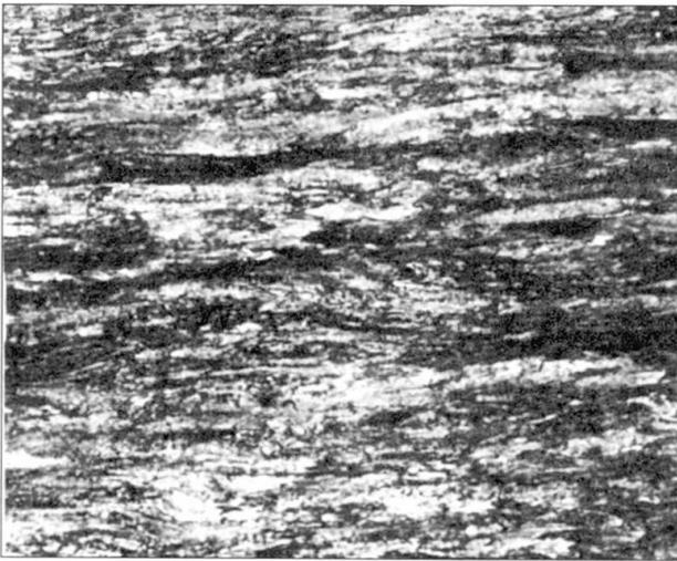
Fig. 10 Micro-Structure of a Galvanized Wire (400 Magnifications)
