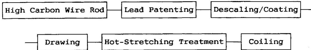
Fig. 1 Diagram for Manufacturing Method for Prestressing Wire
