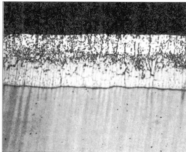
Fig. 11 Micro-Structure of Zinc Coating (400 Magnifications)
