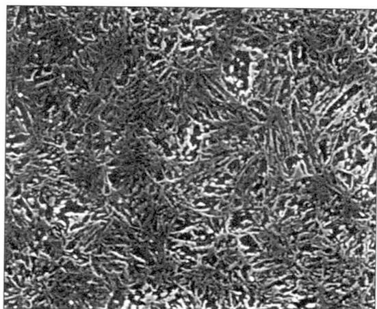
Fig. 6 Micro-Structure of an OT Wire (5,000 Magnifications)
