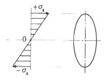
(A) Stress Cycles in a Rotating Bending Fatigue Test
