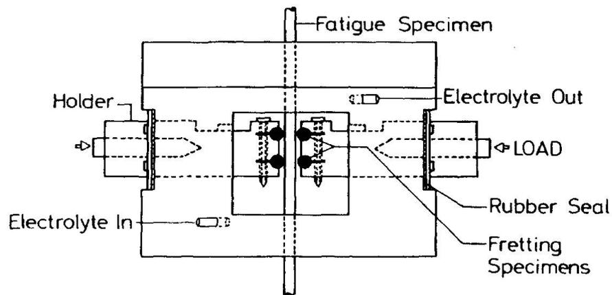
Fig. 2 Experimental rig for testing steel wires under fretting conditions.
