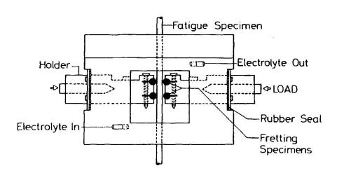
Fig. 2 Experimental rig for testing steel wires under fretting conditions.
