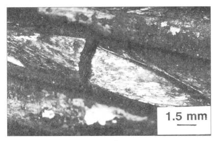
Fig. 1 Failure in a wire due to fretting at a trellis contact.
