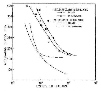
$\underline{\text{Fig. 4}}$  Fatigue curves for hot-dip galvanised wire in air and seawater under fretting conditions.
