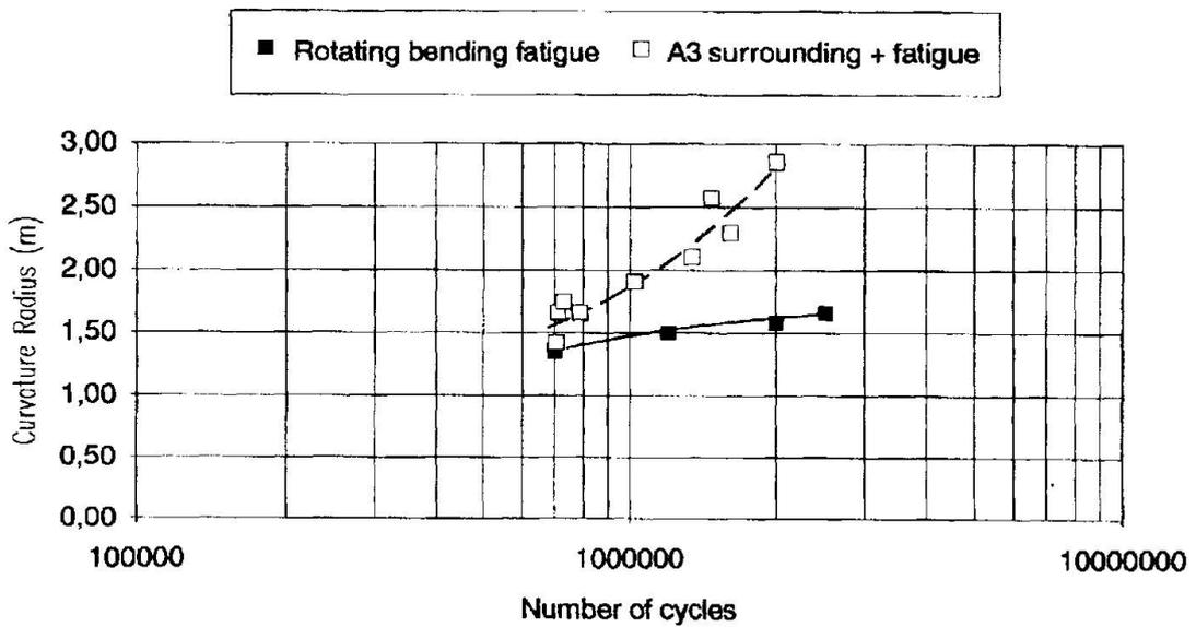
Fig.4 Results on galvanized strands 12.6 mm diameter
