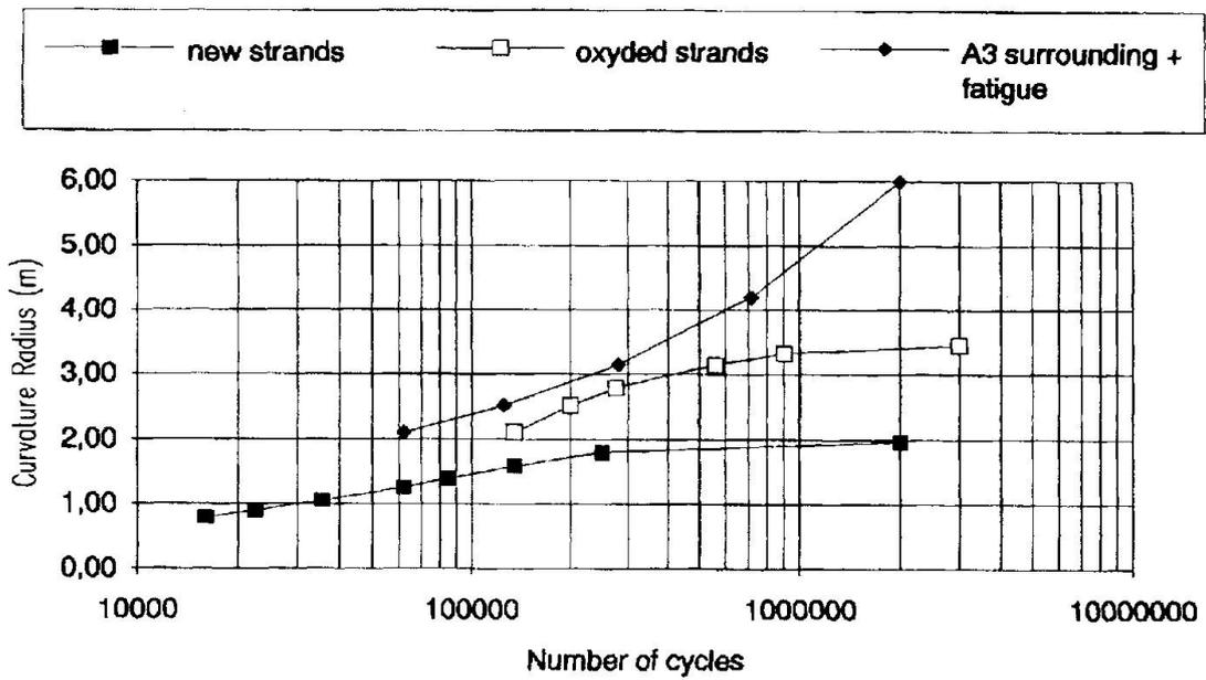
Fig.3 Results on non-coated strands 12.6 mm diameter
