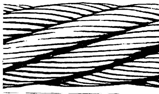
Fig. 11 Roebling's first round stranded cable with 7 x 19 regular lay and a diameter of approx. 30 mm, Saxonbourg, Pa. (1842) [21]
