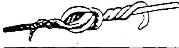
Fig. 9 Wire knot according to Marc Seguin (approx. 1820) Annonay [18]
