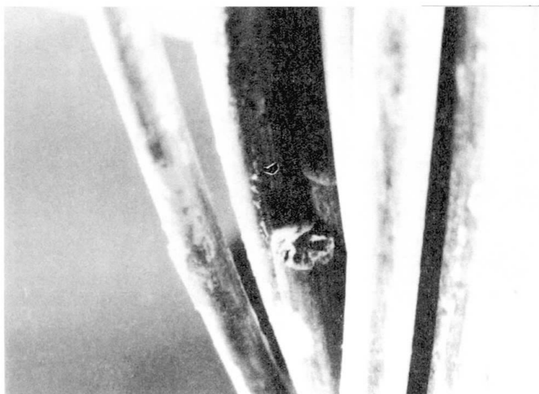
Fig 7 Fretting fatigue in 19-wire strand.
