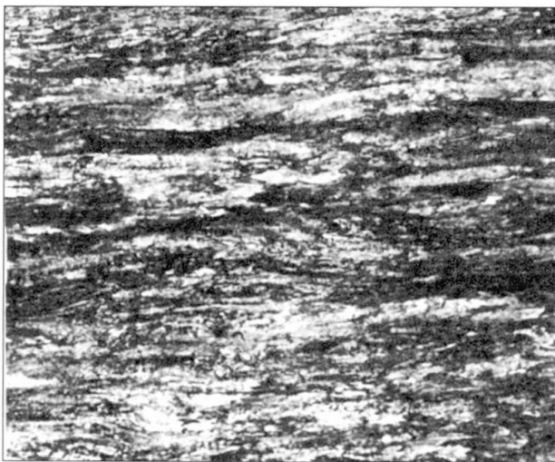
Fig. 10 Micro-Structure of a Galvanized Wire (400 Magnifications)
