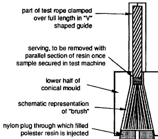
Figure 1: Arrangement employed for moulding conical ends of test samples, injecting resin vertically upwards into the mould.
