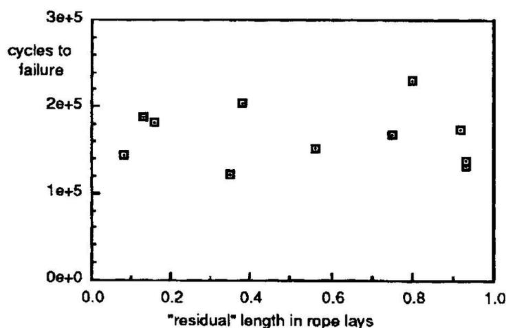
Figure 3: Valid test results plotted in terms of "residual" length, defined as the remainder of length between socket faces, in rope lay lengths, after subtracting the integral part of the length.
