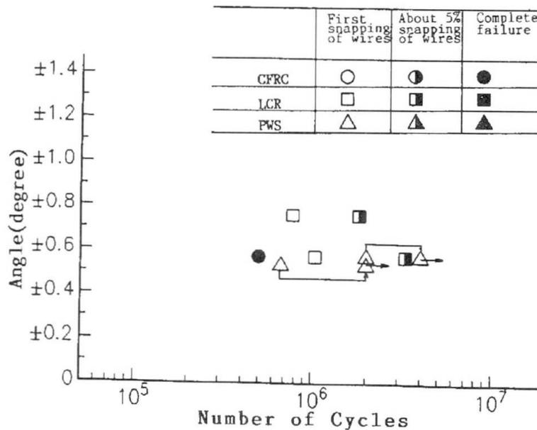
Fig. 12 Results of bending fatigue test (I)
