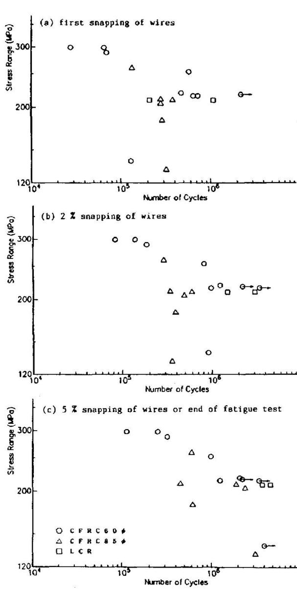
Fig. 7 S-N relationship of CFRC60, CFRC85 and LCR
