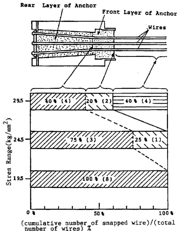
Fig. 5 Locations of wire breakage in HiAm cable systems
