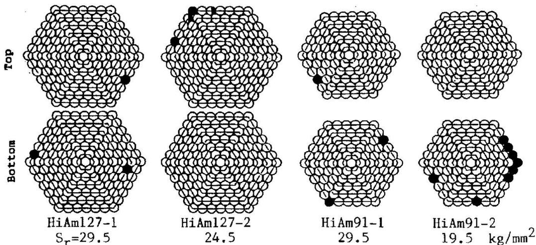
Fig. 6 Positions of snapped wire in HiAm cables
