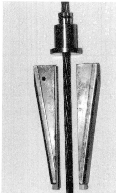
**Figure 4:** Clamping system for the 0.6 inch strand
