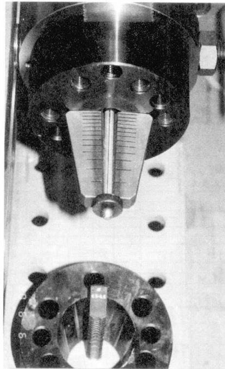
**Figure 3:** Clamping system for the 7 mm prestressing wire
