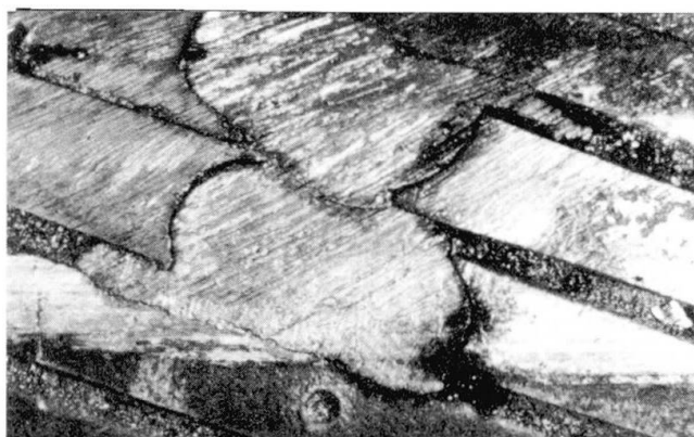
Fig. 8: The minimal gap between the wires and the lead filling shows that the stress of the two adjacent broken wires has not been relieved because of the passage of loaded rollers (d) and because of a track rope braking (e). Data of the braking: Shoe lining material = multicomponent bronze; shoe length 260 mm; shoe pressure 90 kN.
