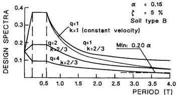
Fig. 3 Design Spectra for different behaviour factors q
