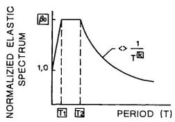
Fig.1 General shape of the normalized elastic response spectrum
