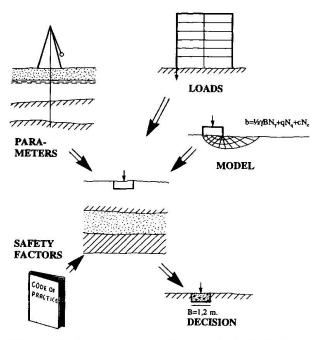
Figure 1. Components of geotechnical design
