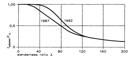
Figure 2 Comparison between the buckling strength of glued laminated columns according to the 1992and the 1987-version (solid line). From [8]. The column strength is  $f_{\text{column}}$ ,  $f_c$  is the compression strength.
