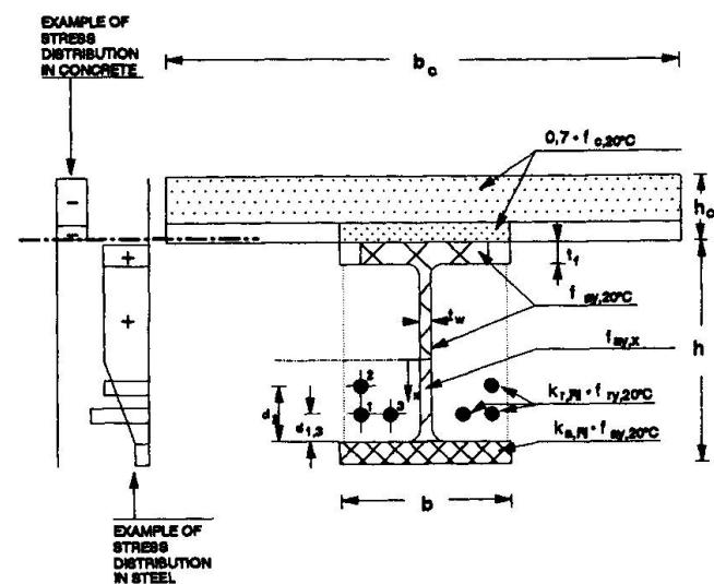
Fig. 6 : Evaluation of the positive plastic bending moment resistance of a composite beam, for different ISO-fire classes R30 to R180 (LEVEL 2).
