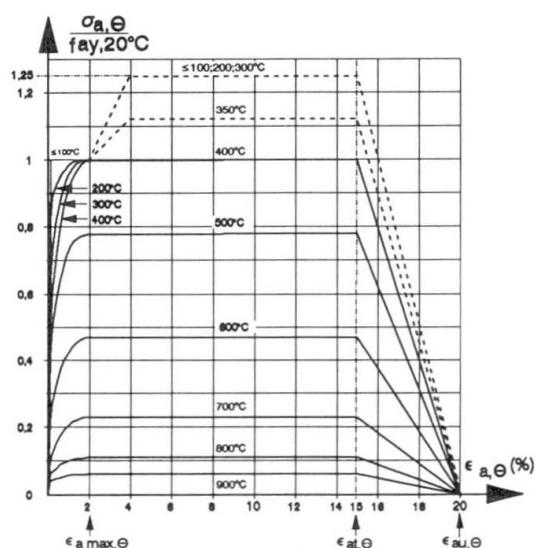
Fig. 2 : Stress-strain relationships for steel at high rising temperatures.
