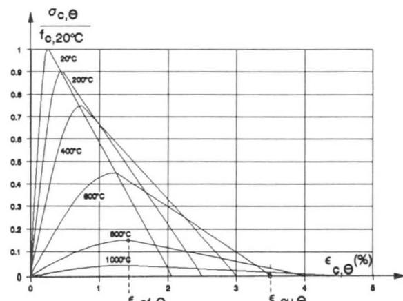
Fig. 3: Stress-strain relationships for concrete at high rising temperatures.
