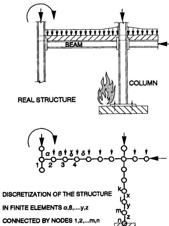
Fig. 7 : Real structure with discretization in finite elements.
