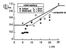
Figure 3 Minimum degree of shear connection for ductile connectors
