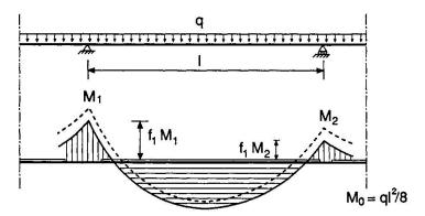
Figure 1 Simplified method for control of deflection
