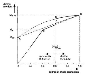
Figure 2 Design diagrams for partial shear connection
