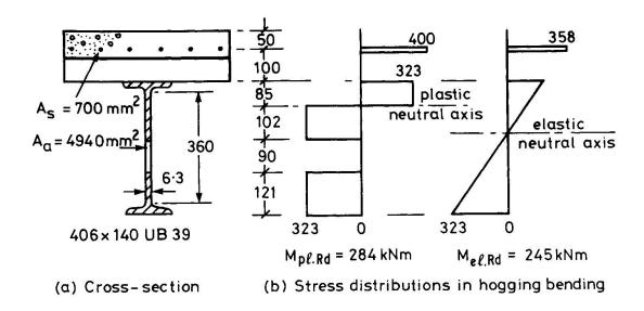
Fig. 1 Replacement of a Class 3 web by an effective web in Class 2
