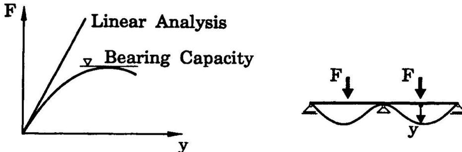
Fig. 5 F-y-Relation for Linear and Nonlinear Design
