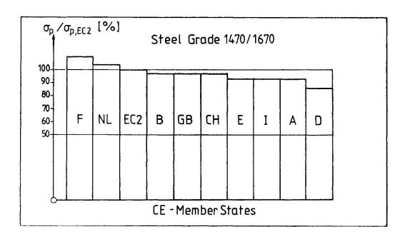
Fig. 3: Comparison of the admissible stresses  $\sigma_{\mathbf{p}}$  in prestressing tendons
