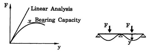
Fig. 5 F-y-Relation for Linear and Nonlinear Design
