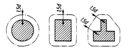
Fig. 3 Perimeters for punching
