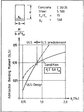
Fig. 8: Link between ULSand SLS conditions in the design concept of EC2
