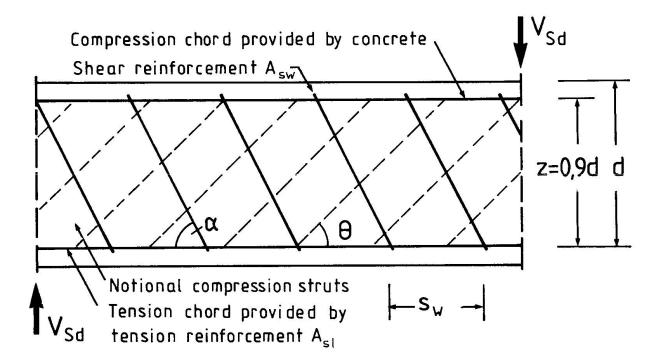
Fig. 2 Assumptions for the calculation of shear reinforcement
