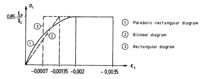
(b) Concrete design stress-strain curves
