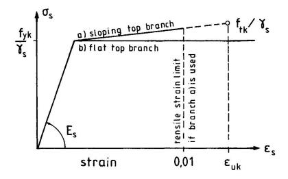
(a) Design stress-strain curves for reinforcement
