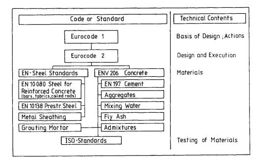
Fig. 1: Future Regulation System for Concrete Structures
