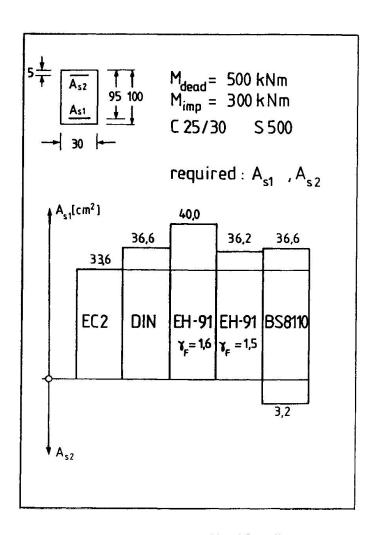
Fig. 7: Comparison of Design Results according to EC2, DIN 1045, BS 8110 and the Spanish Code EH-91
