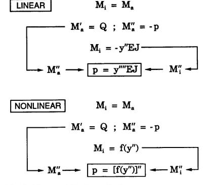
Fig. 3 Linear and Nonlinear Design
