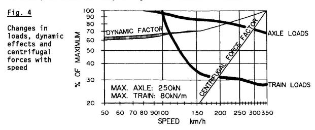
The two lines from left to right show how axle and average train loads drop from their maximum values as speed increases. Values for bending moments on various spans will lie between these lines.
