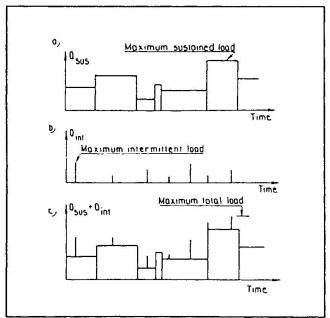
Figure 3: Sustained load (Q<sub>sus</sub>), intermittent load (Q<sub>int</sub>) and total load as stochastic process representing the variability
