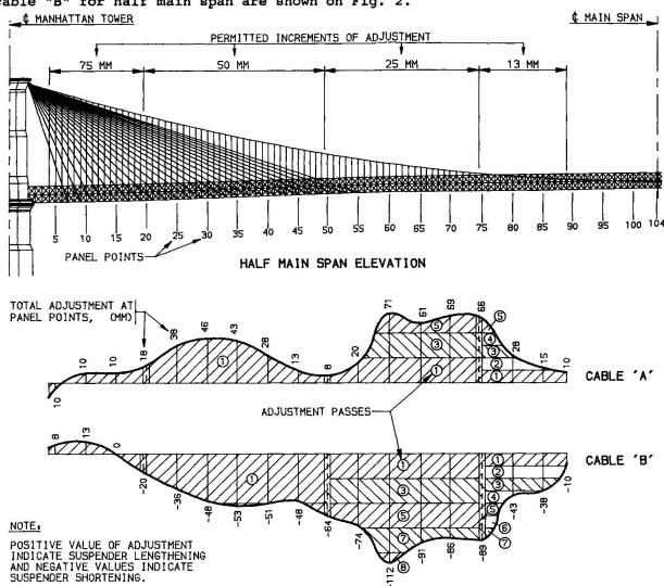
Fig. 2 Adjustment passes. Brooklyn half of Main Span
