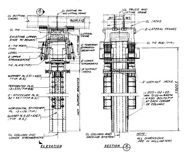
Fig. 4 Bearing replacement jacking system.
